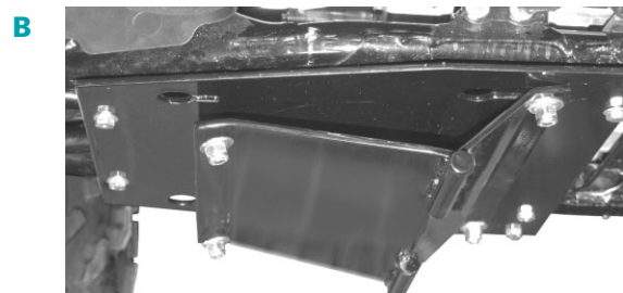
Part B, the Universal tube frame mount, is attached to the mounting plate with four carriage bolts. Easy to install or remove within a few minutes.
