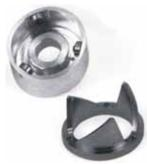
The ultimate in clutch action for your PVT. The plastic buttons and aluminum cam are replaced with ball bearings and a steel cam. The friction-free shifting action gives you immediate response to changing load conditions and improves both acceleration and throttle response on hills and in tight corners. Direct bolt-on, no machining needed.
